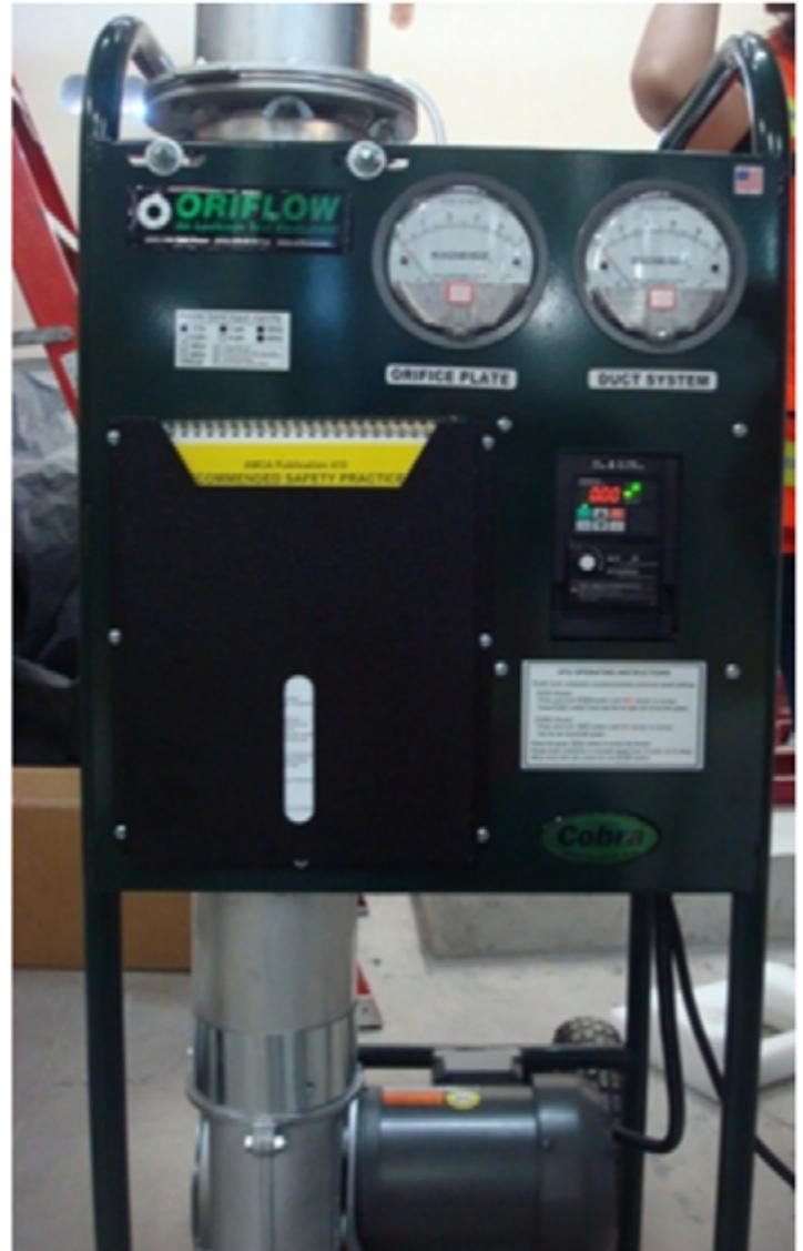
**ORIFLOW (Air Leakage Test Equipment)**
